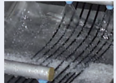
Well-designed details – rounded start-up head to prevent the deposit of polymer strands
