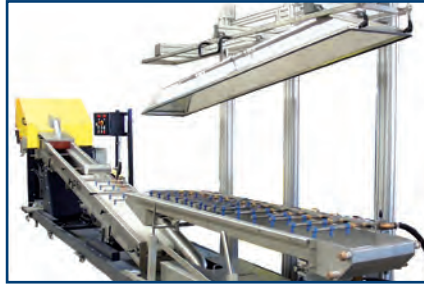
Extraction above the strand cooling chute
