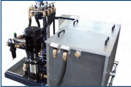
Process water system with filtering and temperature control
