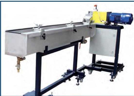
Strand pelletizer with integrated strand cooling trough 2 to 4 m in length with the option of efficient strand drying by blowing (standard) or suction;
