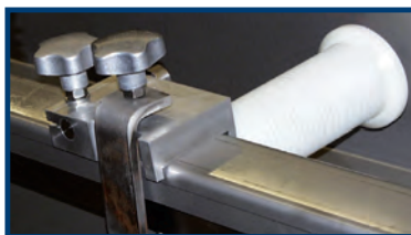
Strand guide roller mounted on one side for optimum accessibility
