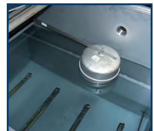
Process water tank with heating and automatic fill level control
