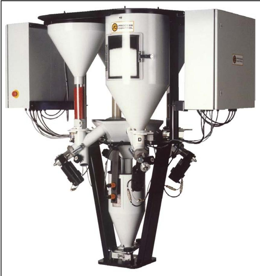
*The X-Series: designed to produce precise, homogeneous blends by weight (pictured is a XGG4)*
