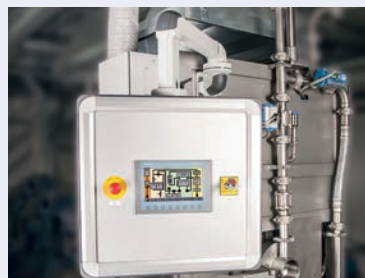
Swivelling control panel
